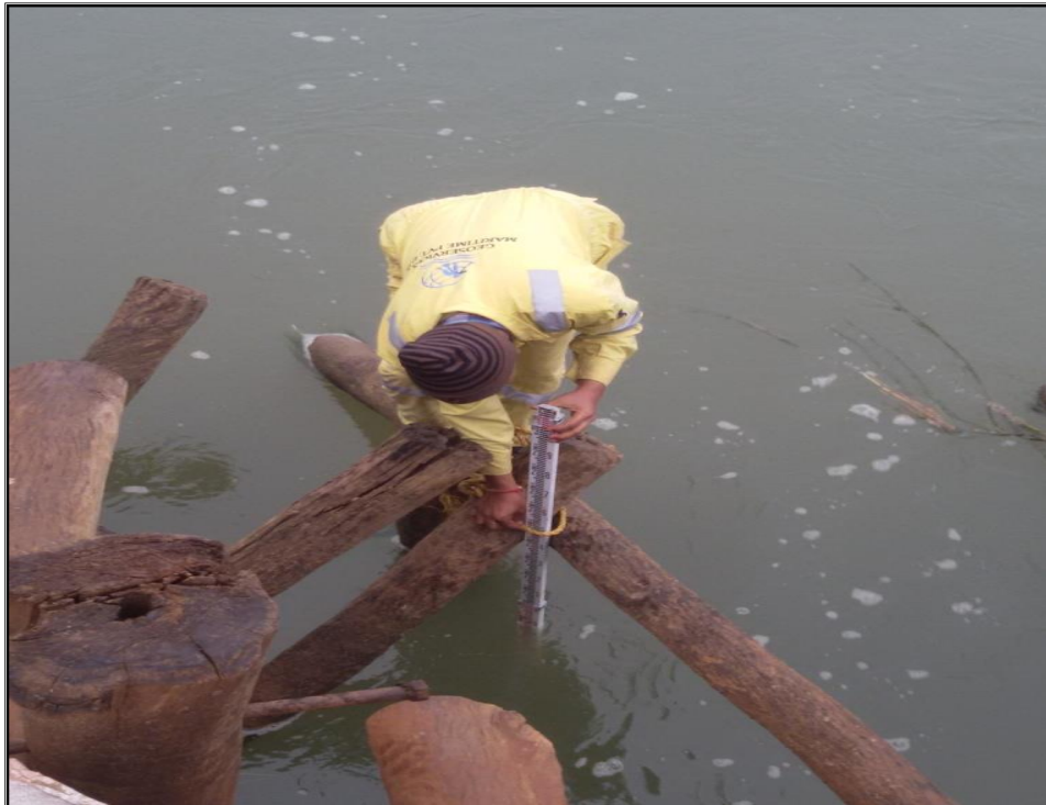
TIDE POLE ERECTED AT SONAKANIA
