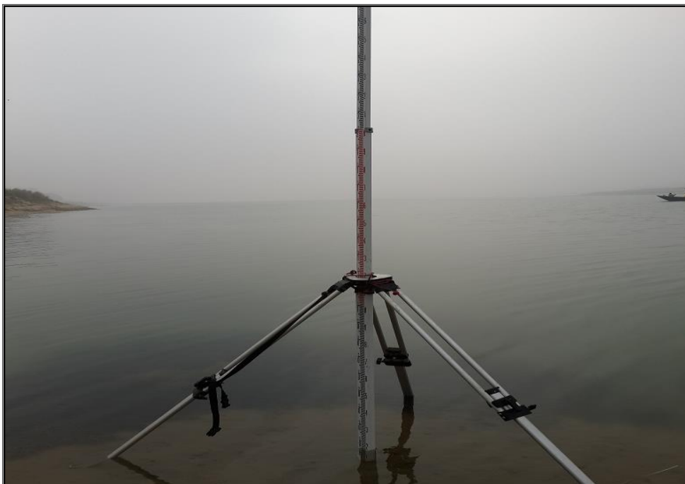
TIDE POLE ERECTED IN WATERWAY
