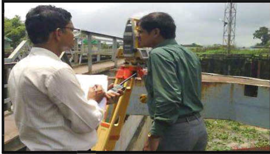
Total station survey at Farakka land area
