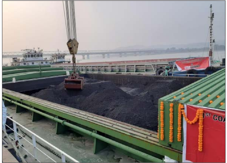
Figure 24- NW-2: Coal handling operations at Pandu terminal
