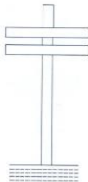
BATH (LEFT HAND MARK) LEAVE LEFT SIDE WHILE COMING RIGHT AND UP STREAM
